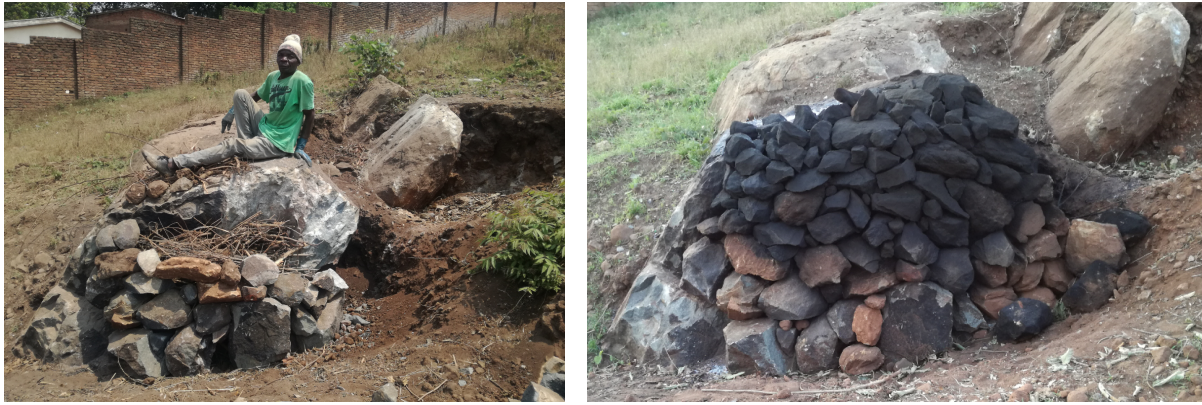
Figure 4. Excavation and heating procedure (Left: unburnt; Right: burnt)
